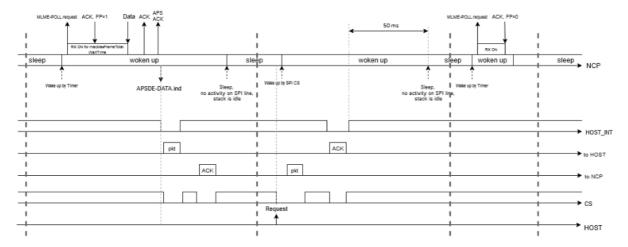
Host introduces some delay between CS line activation and starting packet transmission. During that time NCP finishes its wake-up (if occurred) and preparation for transfer and is able to receive the packet from Host.
